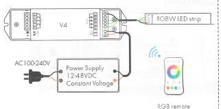
Note: If connect with RGB LED strip, please long press match key for 15s, the controller will become RGB type, the LED indicator blinks 2 time. (Long press match key for 10s will restore to RGBW type)
