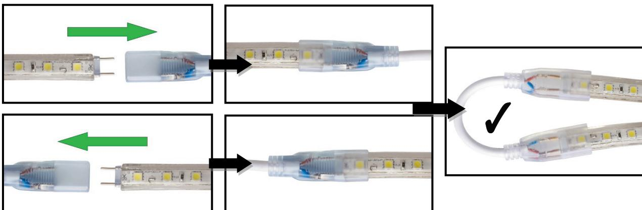
**Important:** For wet locations, seal the connection with silicone sealant and cover with glue lined heat shrink tubing (see 'waterproofing connections').
