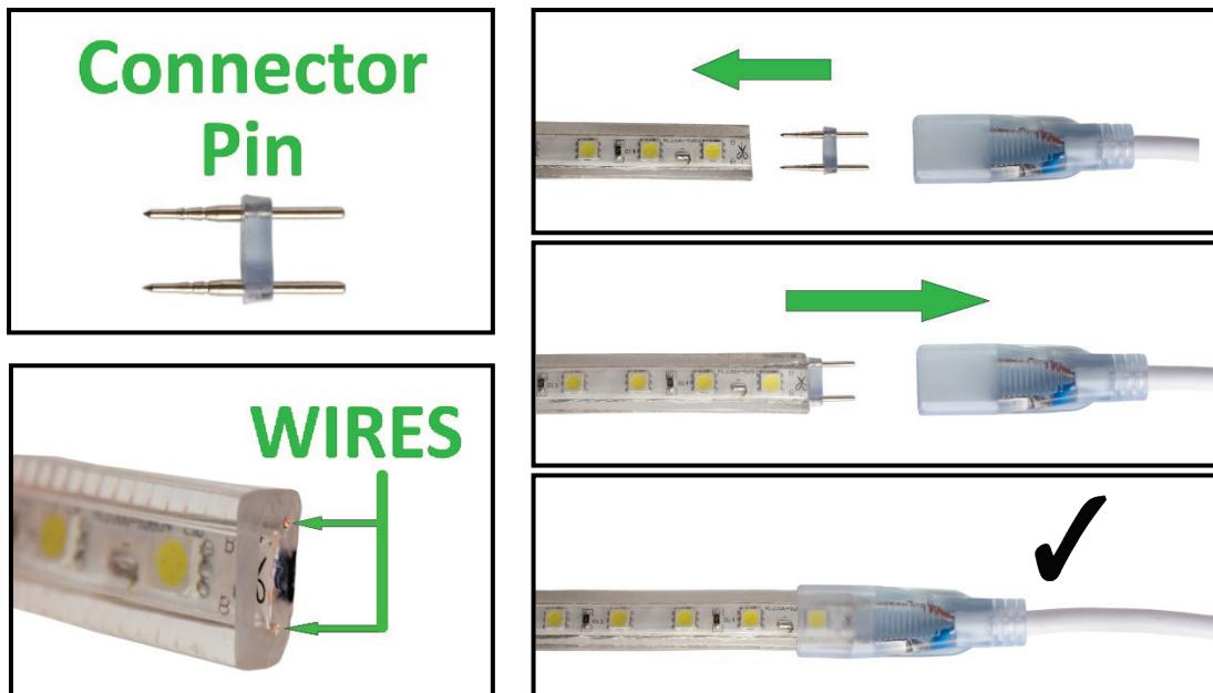
**Important: For wet locations, seal the connection with silicone sealant and cover with glue lined heat shrink tubing.**
